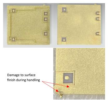
Proper handling and care should be observed to preserve the gold finish and wire-bondable surface refer to the "Handling and Storage" section for more information.
