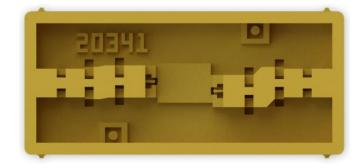
The typical use case includes size 1515 single layer, wirebondable 100 pF capacitors in this area to filter gate and drain signals. Any additional components for signal conditioning would be located on the PCB, outside the package.
